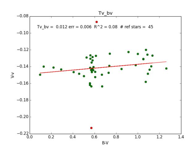
From this plot we extract the slope of the curve. This number, the transform coefficient, quantifies how your system is different and we will apply it to your observations to get to the standard framework.
