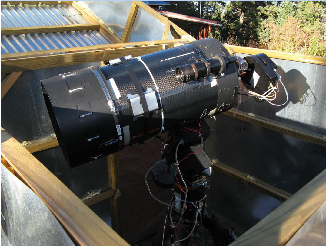
SBIG ST-7XME CCD Camera Pixels binned 2x2 to give 382 x 255
