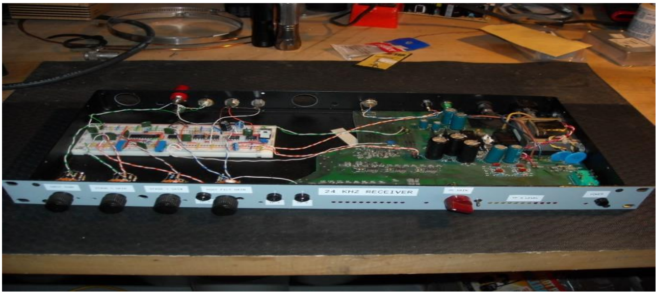
Picture above is what the 24 kHz receiver looks like in the rack box, it is designed with multiple stage amplifier gain switches for the audio, and the red knob is for DC gain.
